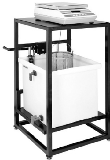
Figure 9: Specific Gravity and Absorption Device
