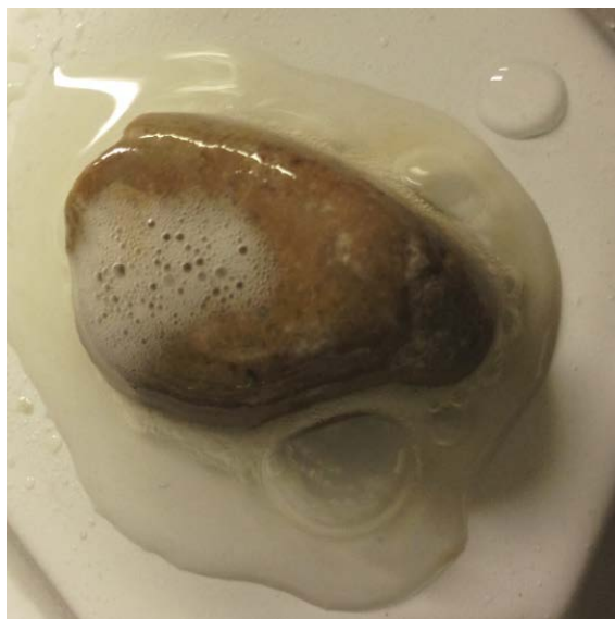
Figure 6: Carbonate Aggregate Surface React with Acid Solution
